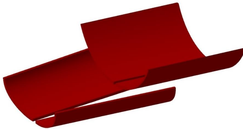
Figure 14 - Radiators volume for CS-25 80-passenger aircraft.
