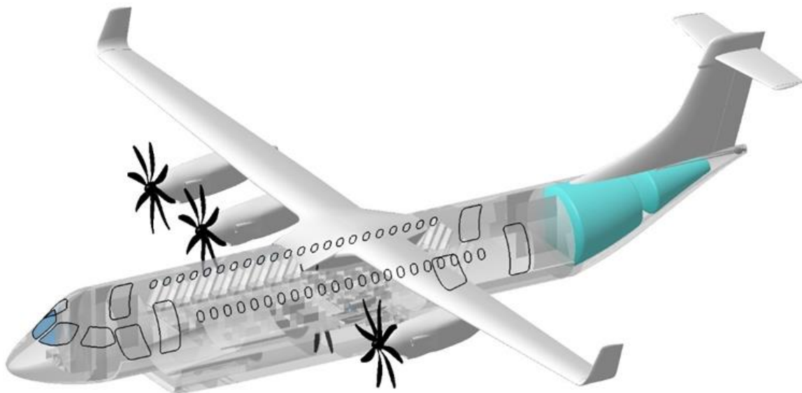
Figure 17 - Integrated representation of fuel tank within CS-25 80-passenger aircraft.
