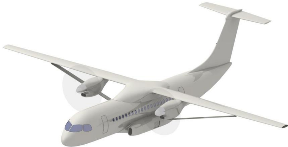
Figure 9 - CS-25 HERA airframe.
