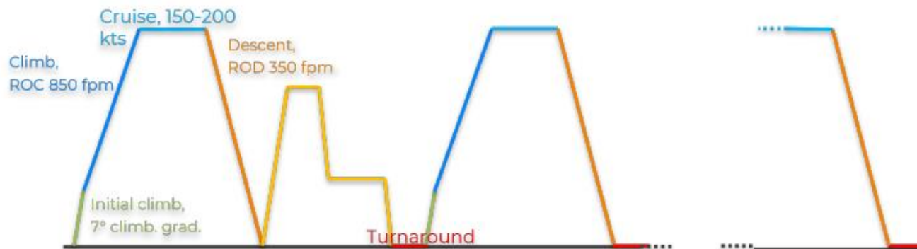
Figure 2: 5-hop mission profile of the Pipistrel Miniliner. Source: UNIFIER19 project.
